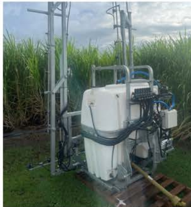
Seven row seven section flatboom with Isobus rate control and Swath control
